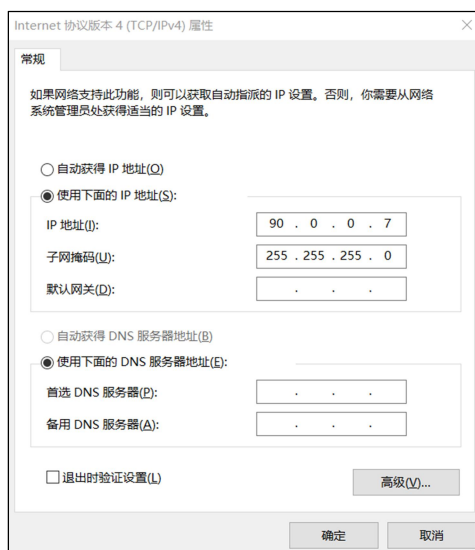
Figure 2-3 Network Setting for PC Connected to Controller
