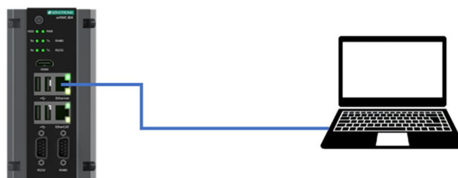
Figure 2-2 Controller and PC Connected via Network Cable
