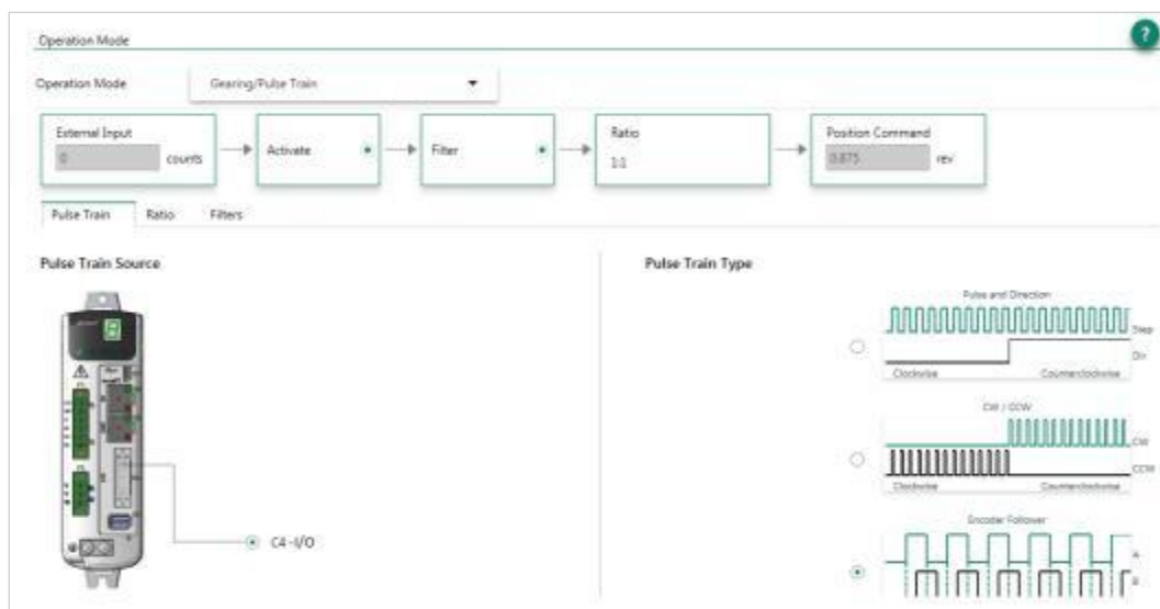
figure7-8 Settings for Pulse & Direction Commands
