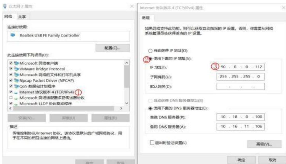
Figure 2-4 Network Setting for PC Connected to Controller
