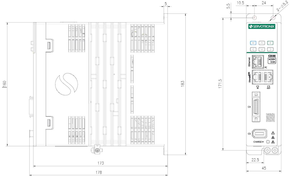
Figure 3-1. CD3E-003 Dimensions (mm)
