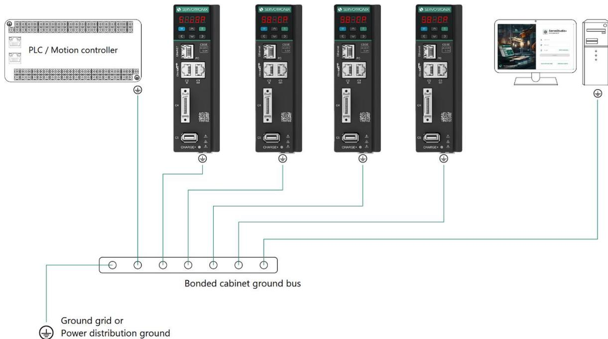
Figure 4-4. System Grounding
