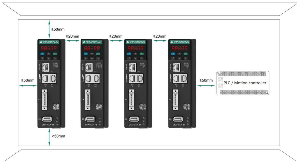
Figure 4-1. Mounting Multiple CD3E Units within Cabinet
