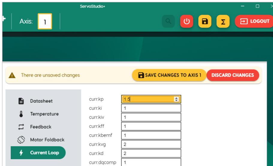
Figure 7-2. Save changes to axis (saves parameter in drive)
