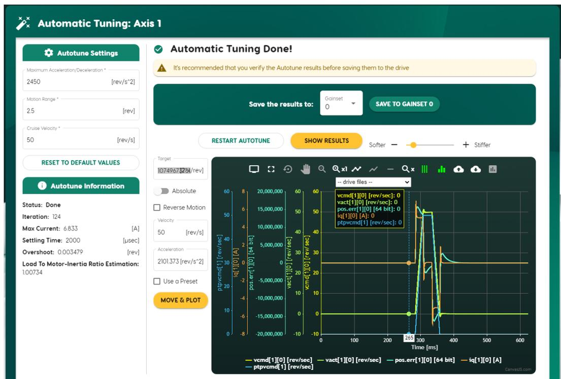
Figure 7-6. Autotuning test results
