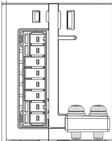
Figure 4-2. PE terminal screws
