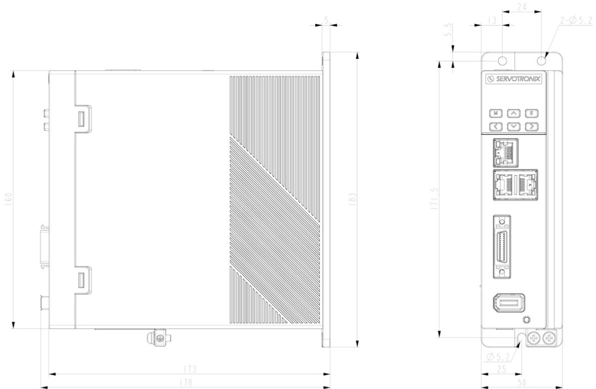
Figure 3-2. CD3E-5D5 Dimensions (mm)
