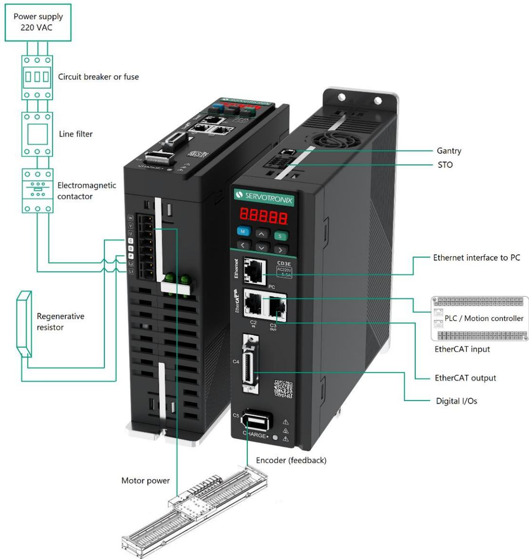
Figure 4-2. System Wiring
